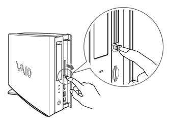
When the PC card is ejected from the card connector, remove the card by holding the edges and pulling it out carefully.
